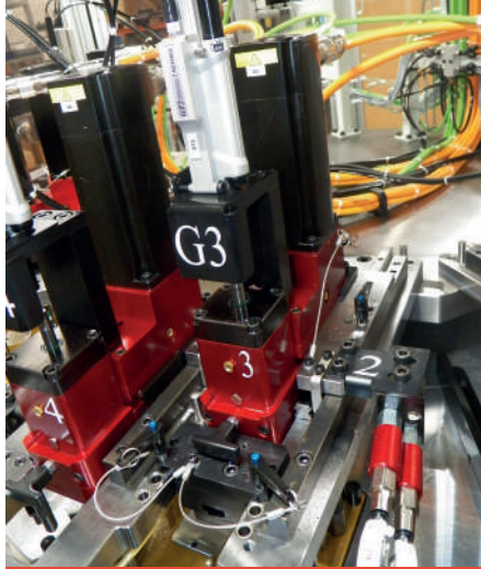
Tap detection (guaranteeing 100% tapped holes)
