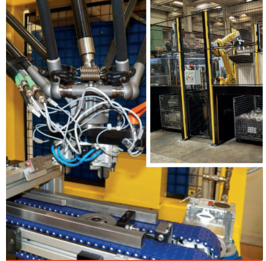
Robot loading from bulk containers.
