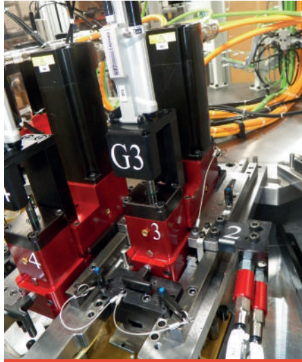
Tap detection (guaranteeing 100% tapped holes)
